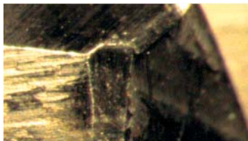
Tooth chamfering after chamfer, Nital tested, Ferrite structure with a 25% Pearlite portion, compressed due to the pressure exerted by the chamfering tool
