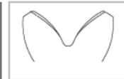
Comma type chamfer of both flanks without chamfering of the root radius
