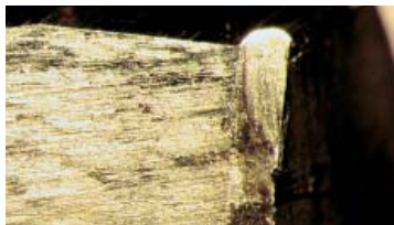
Tooth chamfers after chamfering and rolling, Ferrite structure with a 25% Pearlite portion, compressed due to the pressure exerted by the chamfering tool
