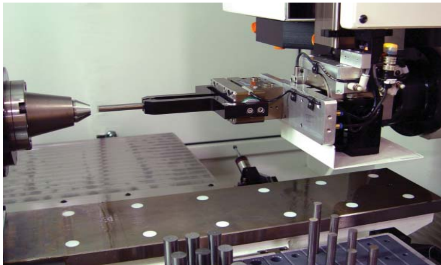
PTG6 with optional Pick & Place automated loader with pallet.
