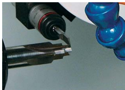
Round tools are manufactured and resharpener in the same CNC equipment.
